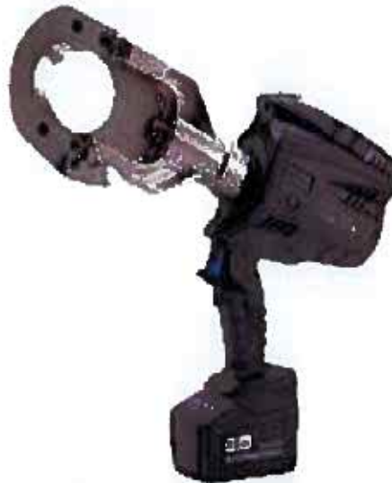
Figure 2: Typical Cordless Battery Hydraulic Cutting Tool
