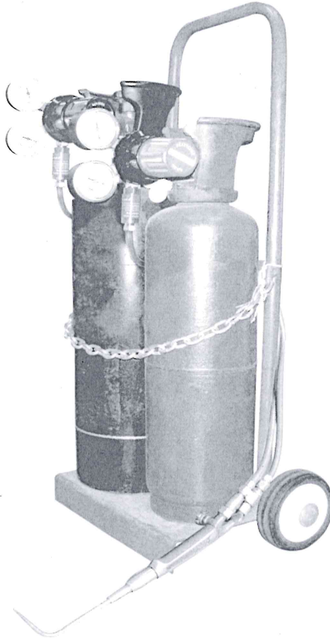
Figure 6: A typical pair of oxygen and acetylene cylinders in a wheeled rack for portability
