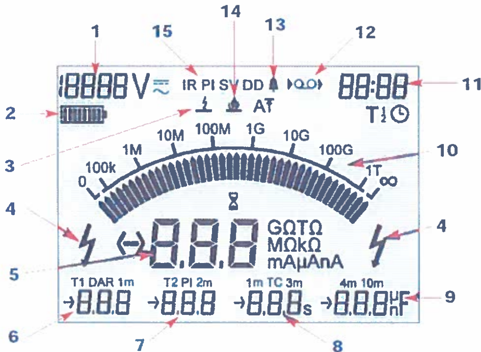
Fig. 2: Typical Insulation resistance digital display.
