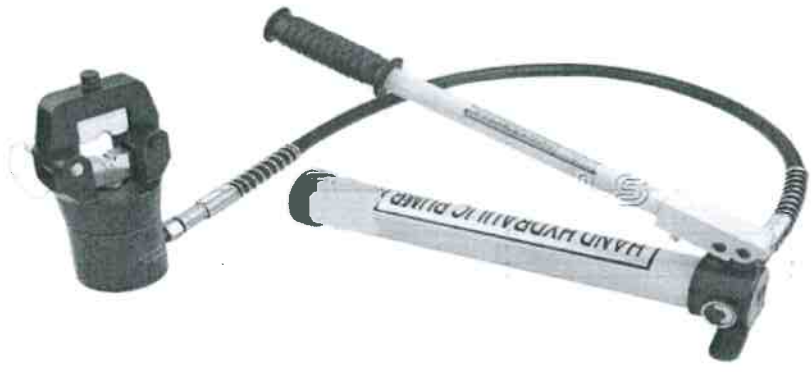
Fig. 5: Typical Split Hydraulic Cable Jointing Tool Kit
