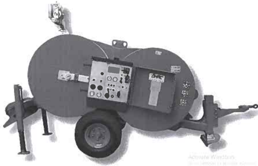
Figure 1: Typical Hydraulic Puller Tensioner Stringing Equipment
