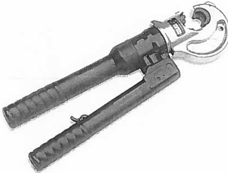
Fig. 3: Hand Operated Hydraulic Compression Tool of up to 300mm 2
