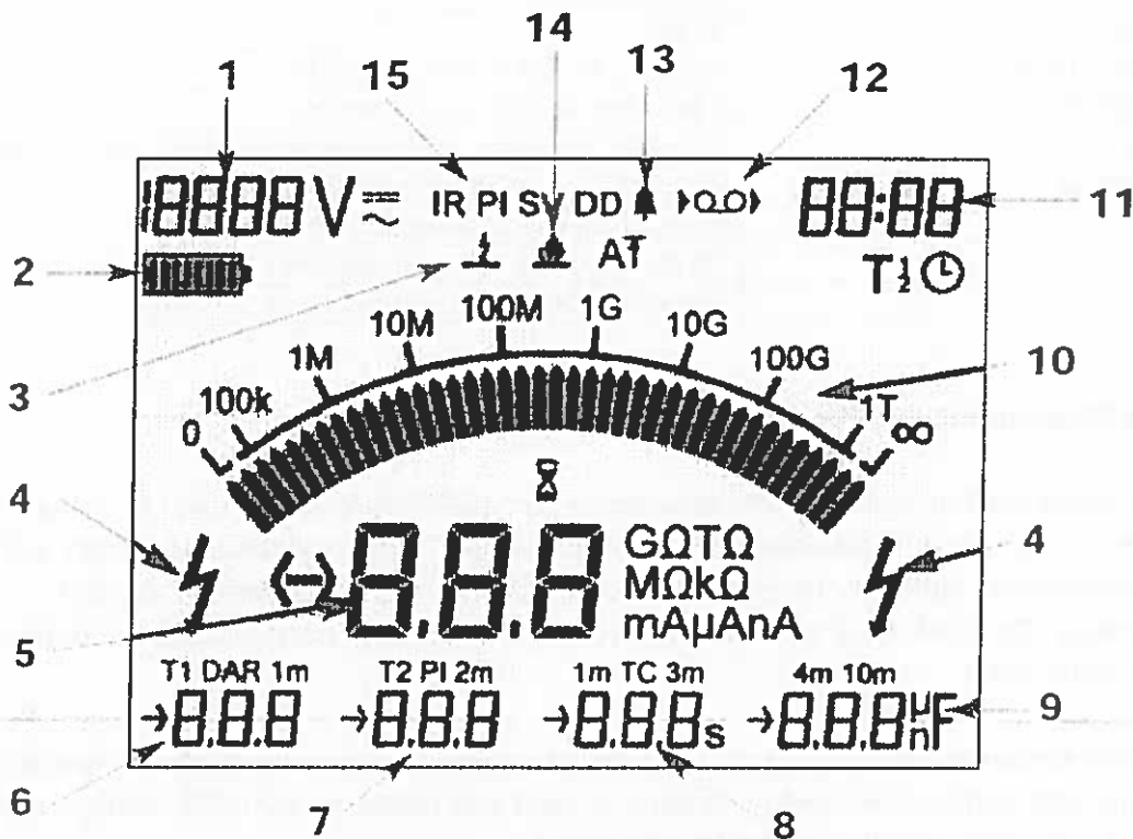
Fig. 2: Insulation resistance digital display.
