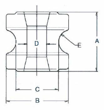
Fig. 1: A typical low voltage insulator (shackle insulator)
