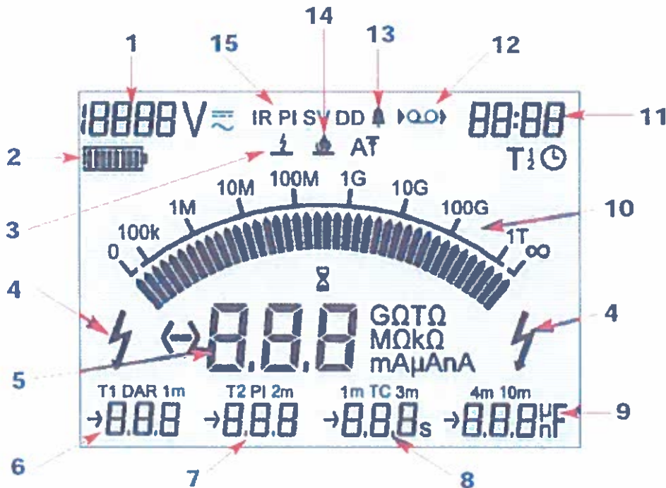
Fig. 2: Typical Insulation resistance digital display.
